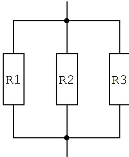
$$\frac{1}{R_G} = \frac{1}{R_1} + \frac{1}{R_2} + \frac{1}{R_3}$$
